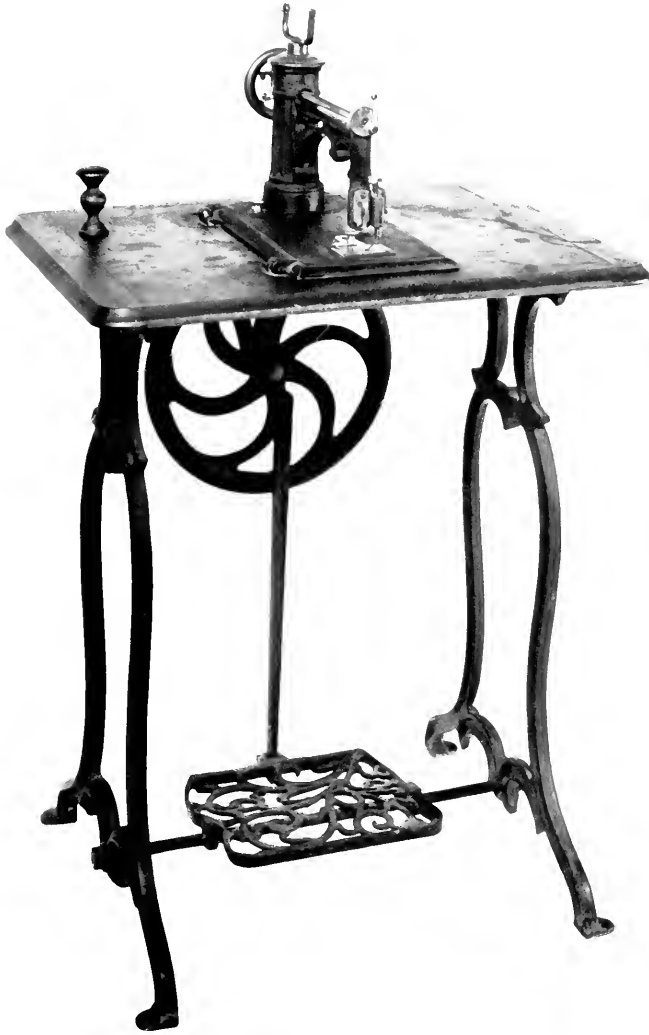
Figure 127.—WEST & WILLSON SEWING MACHINE of about 1859. The West & Willson machine, manufactured under the patent of H. B. West and H. F. Willson, enjoyed a very brief span of popularity. The patent covered the peculiar method of operating a spring-looper in combination with an eye-pointed needle to form a single chainstitch, but whether
